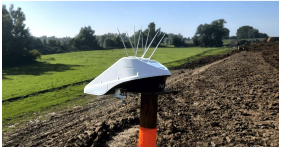
Locator One sensor mounted on settlement plate riser pipe and protected by bird spikes
